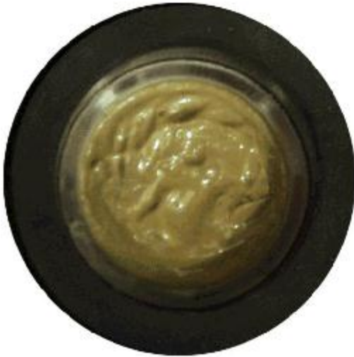
Figure 8 – Photograph of Filtercake showing imprint of outer expandable screen shroud pressed into filter cake prior to flow-back Before After
